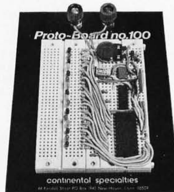
Proto-Board® 100. 760 solderless tie-points. Kit, $19.95*
